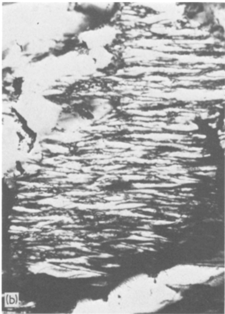
Figure 5 Dynamic recrystallization originating at deformation twins during deformation at 293 K. (Compression axis vertical.)
