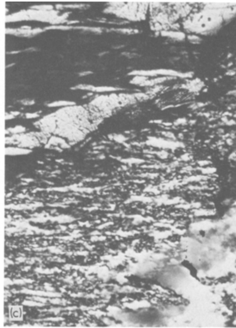
Figure 5 Dynamic recrystallization originating at deformation twins during deformation at 293 K. (Compression axis vertical.)
