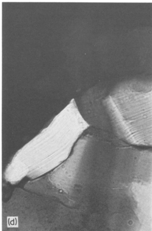
Figure 2 Deformation sequence at 320 K, showing slip, lattice bending, kinking and dynamic recrystallization in the kink bands (compression axis vertical).
